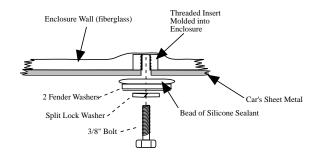
**STEP 8:** While one person holds the Stealthbox in place from above, the other person inserts the bolt, lock washer and fender washers from underneath the vehicle. Put a bead of silicone sealant between the car's sheet metal and the fender washers.
